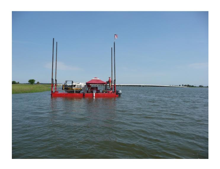
Offshore drill rig used to obtain discrete water samples above the upper confining unit.
